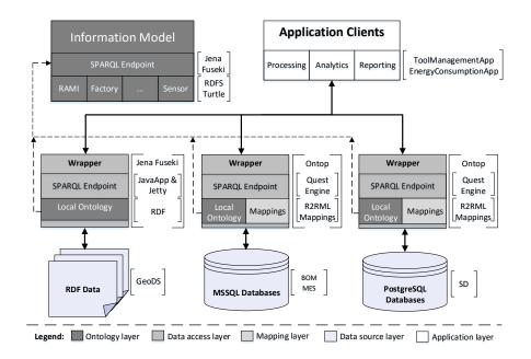
Fig. 3: The implemented architecture comprised of different layers
