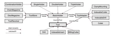
Fig. 2: Ontological view of the Tool concept
